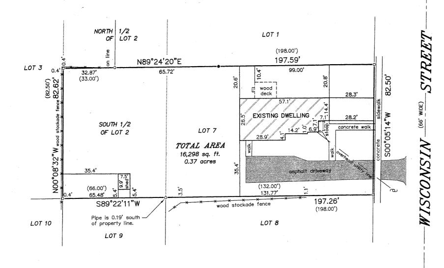
BEARINGS HEREON RELATE TO THE NORTH LINE OF LOT 7 IN BLOCK 18 OF STONE & TOPPING'S ADDITION TO THE VILLAGE OF DARIEN. ASSUMED BEARING OF NORTH 89°24'20" EAST TO ORIENTATE WITH A PREVIOUS SURVEY BY DUNHAM SURVEYING, S.C. DATED NOVEMBER 24, 1992.
